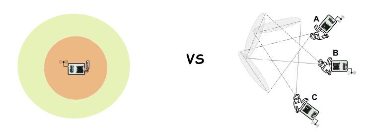
Video sensors capture scene with a Field of View ~ a cone
