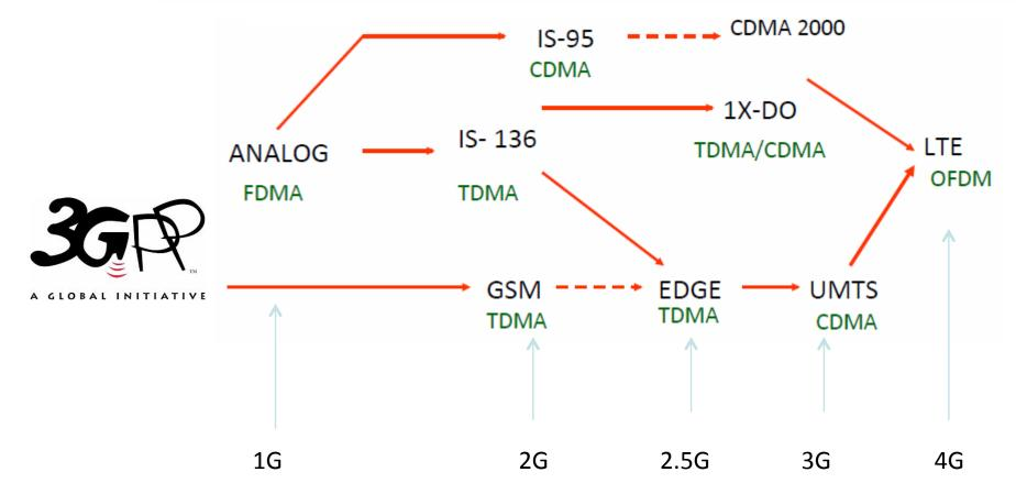
CDMAone->CDMA2000 EGDE: Enhanced Data Rates for GSM Evolution UMTS:Universal Mobile Telecommunications System (W-CDMA)
