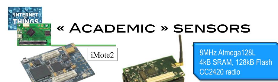
13-416MHz PXA271 Xscale Wireless MMX DSP 256kB SRAM, 32MB 32MB SDRAM CC2420 radio
