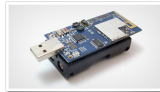
AdvanticSys CM5000 TelosB-like mote
