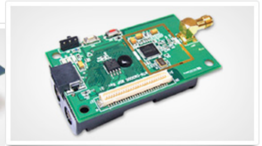
Advanticsys CM5000 & CM3000 TelosB-like mote
