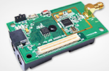
Advanticsys CM5000 & CM3000 TelosB-like mote
