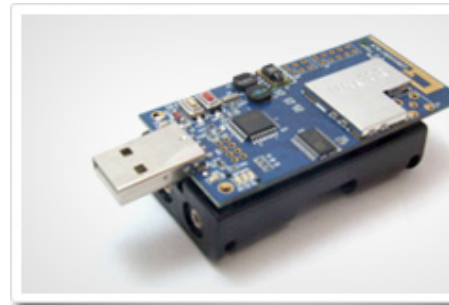
Advanticsys CM5000 & CM3000 TelosB-like mote
