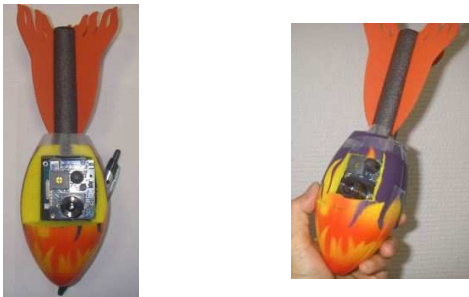
Fig. 1. A proof-of-concept of an image sensor in a beach rocket toy.
