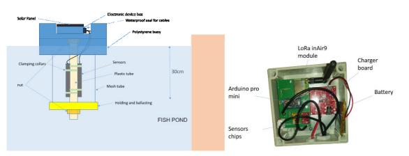
*Figure 3: (a) Schema of the first deployed prototype for aquaculture water monitoring in WAZIUP project. (b) The electronic parts in the waterproof case*
