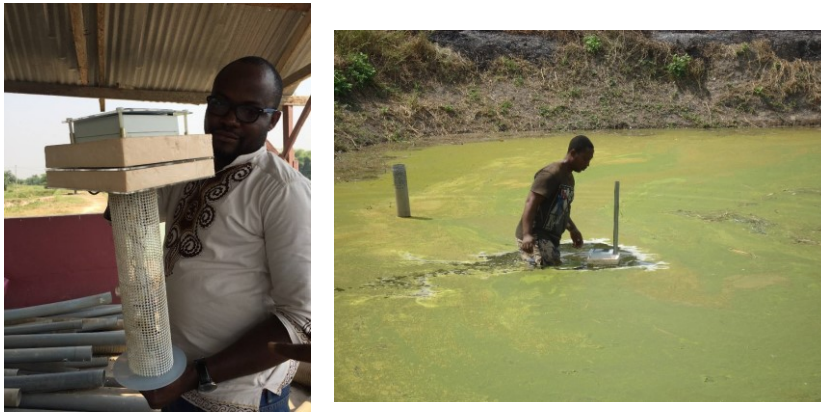
Figure 5 & 6: The prototype low cost buoy and its deployment in fish farm at Kumasi, Ghana
