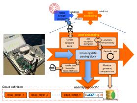
Figure 4. Modular and versatile low-cost gateway
