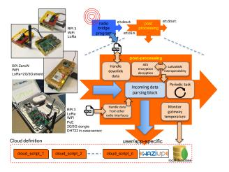
Fig. 3. Modular and versatile low-cost gateway
