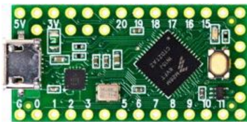
Teensy LC 48 MHz Cortex-M0+ 8K of RAM memory
