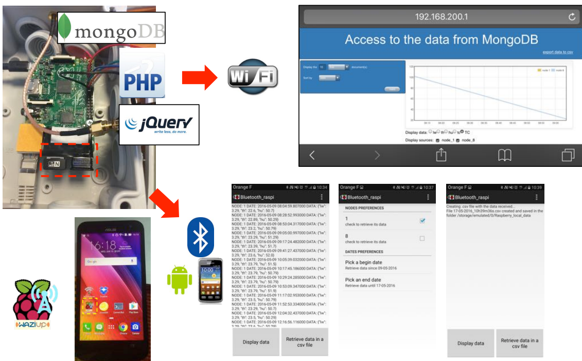
Figure 56 – Autonomous gateway for no-Internet access deployment scenarios
