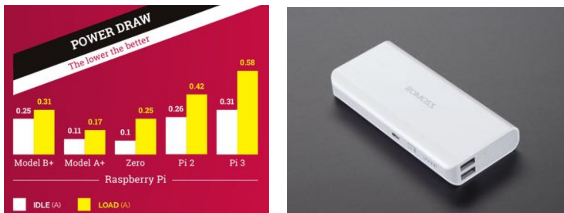
Figure 52 – Raspberry power consumption (left), 10000mAh USB charging pack (right)
