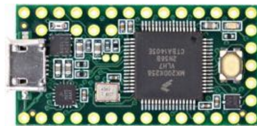
Teensy 3.1 72 MHz Cortex-M4 64KB of RAM memory
