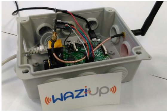
Raspberry PI with LoRa radio module and WiFi
