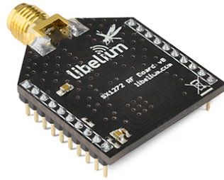
Libelium LoRa is based on Semtech SX1272 LoRa 863-870 MHz for Europe
