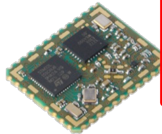
IMST IM880A-L is based on Semtech SX1272 LoRa 863-870 MHz for Europe
