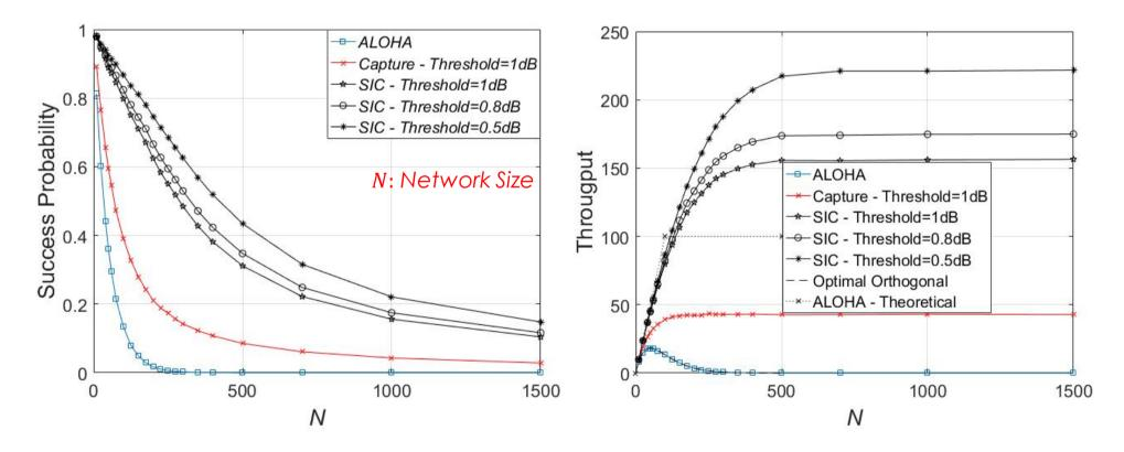
Figure from Umber Noreen, Ahcène Bounceur and Laurent Clavier. LoRa-like CSS-based PHY layer, Capture Effect and Serial Interference Cancellation (24th European Wireless 2018, Catania Italy).
