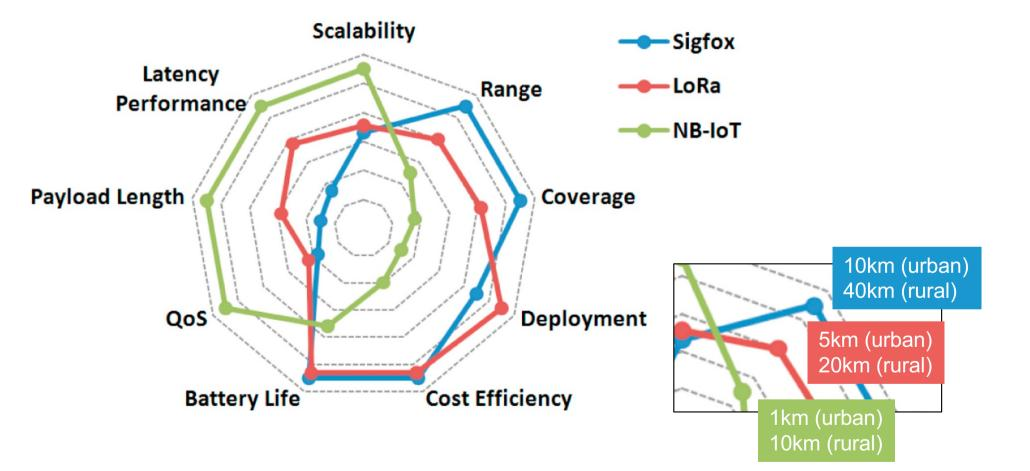
Figure from Kais Mekki, Eddy Bajic, Frederic Chaxel, Fernand Meyer, A comparative study of LPWAN technologies for large-scale IoT deployment, ICT Express, Volume 5, Issue 1, 2019.
