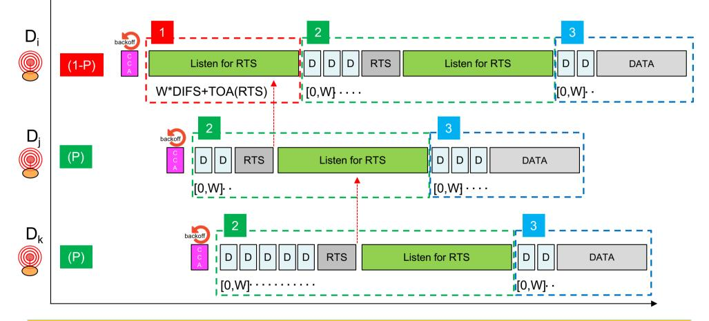
Keep a small proportion of nodes starting directly at phase 2. P=10% for instance
