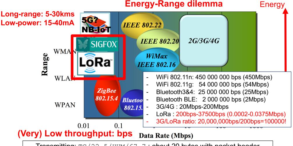
Transmitting: TC/22.5/HUM/67.7; about 20 bytes with packet header Time on air can be 1.44s with LoRa
