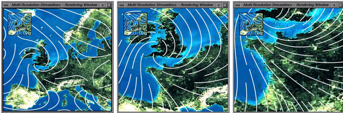
Figure 2: Three snapshots of an interactive exploration of a vector field using our multiresolution viewer. The suitable level of the hierarchy is selected at any time to maintain a roughly constant density of streamlines.
